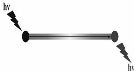
Figure 1: Schematic Representation of an Elementary Photonic "Circuit" (Figure Inspired by Reference [8]).
