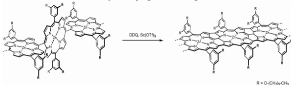
Figure 7: Formation of Bands of Fused Porphyrins from Mesoconnected Oligomers
